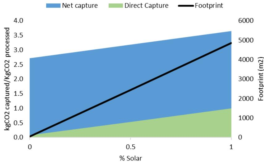
Figure 5- Effect of using PV system to power the process in terms of footprint and CO<sub>2</sub> (for capturing 1200 kg CO<sub>2</sub> per day) balance.
