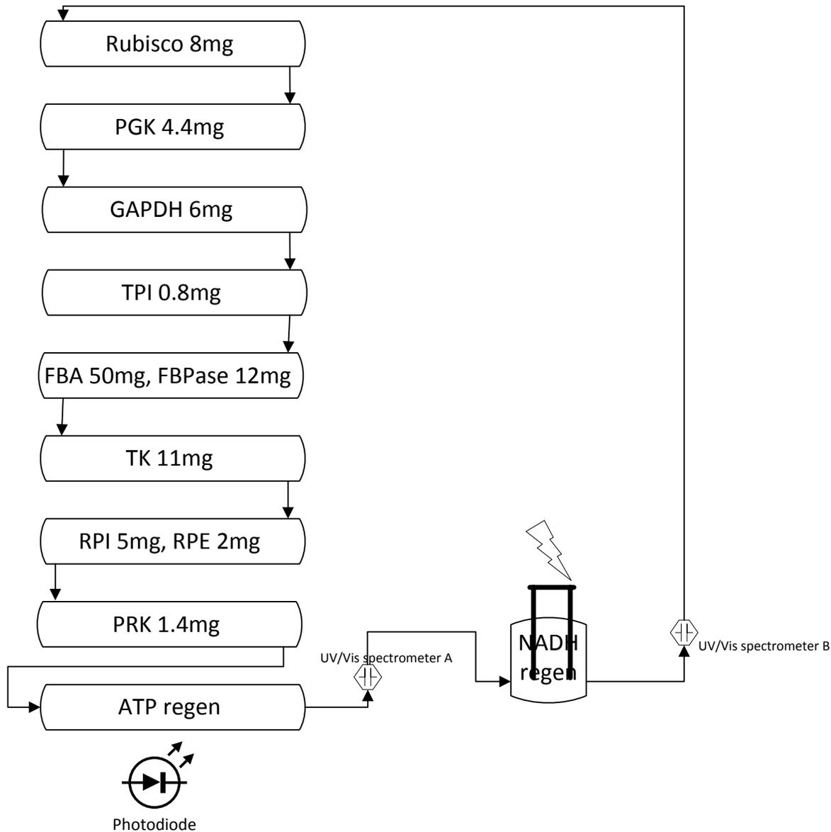
Figure 14- Schematic of the full Calvin cycle experiment
