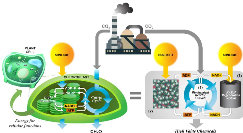
Figure 1- A schematic of artificial photosynthesis mirroring plant cell photosynthesis: (1) Biochemical reactor cascade; (2), ATP regeneration system; (3), NADH regeneration system
