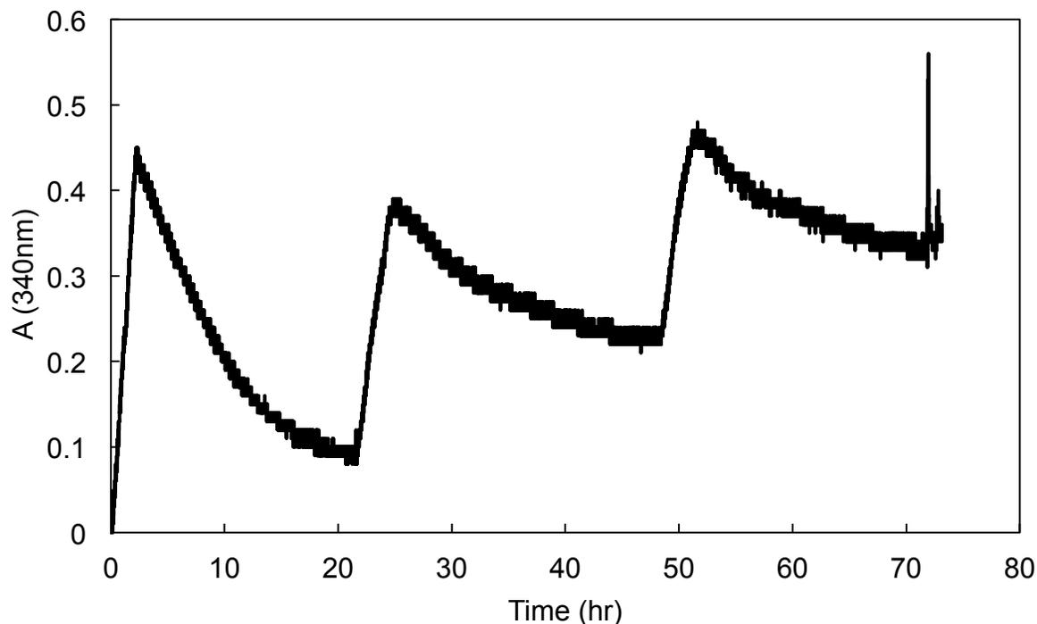
Figure 15- UV/Vis spectrometer trends at 340 nm which corresponds to NADH concentration.
