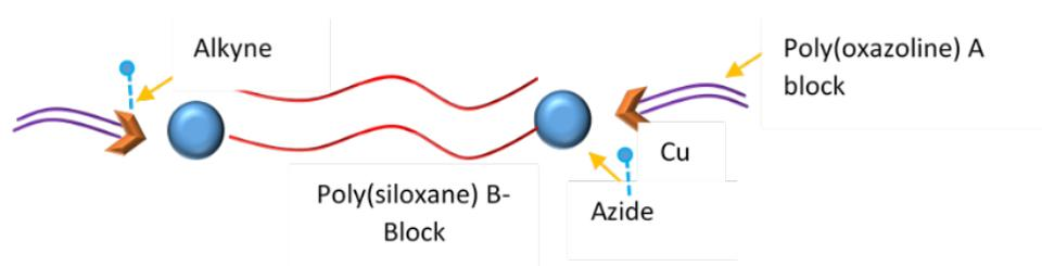
*Figure 9- The A-blocks bear an alkyne terminal group, while the B-blocks are terminated with azides. The two blocks are clicked via a copper-catalyzed azide-alkyne click reaction.*
