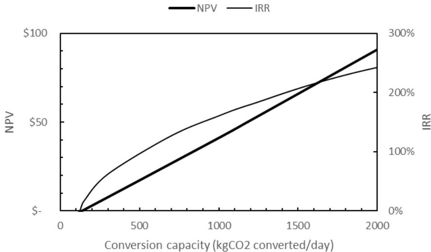
Figure 7- The effect of CO<sub>2</sub> conversion capacity on the economic metrics of the project
